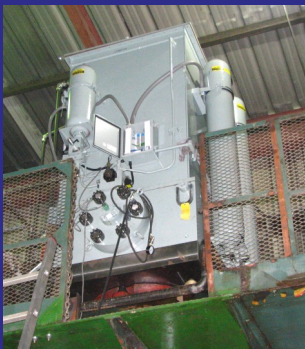
NEW PRESS CONTROL VALVE MANIFOLD AND PREFILL TANK MOUNTED ON THE PRESS CROWN
